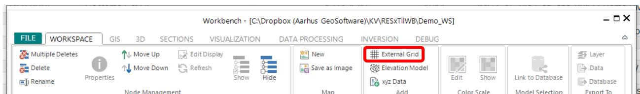
Select the VTK file from Res2/3DInv and select ‘Open’, provide a name for the imported inversion result when prompted and select ‘OK’, select the coordinates system when prompted:
