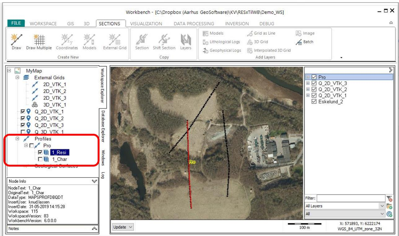
To display the profile, check the checkbox next to it in the 'workspace explorer':
