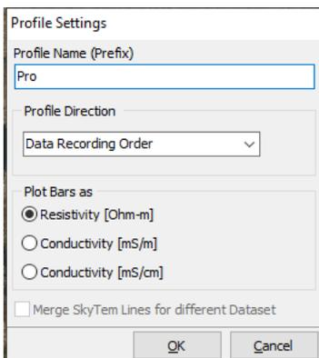
In the next window select from which model selection to add models to the profile, specify the color scale for the different parameters (resistivity and possibly chargeability) and whether to select the models as bars or interpolated sections:
