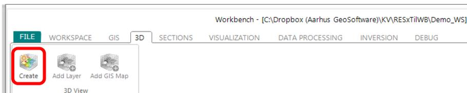
The new 3D view can be found in the Workspace Explorer and opened in a separate window by checking the checkbox next to the name. Objects from the workspace can be added by highlighting them in the Workspace Explorer, navigating to the 3D ribbon and selecting ‘Add GIS Map’ (for GIS maps) or ‘Add Layer’ for everything else. In the below example the background map and 3 model selections have been added to the view:
