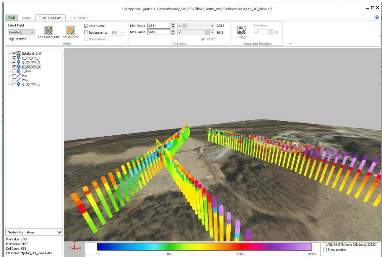
In the example below an inversion result from Res3DInv have been gridded in 3D (Visualization -> 3D grid), added to the 3D viewer and two dipping cut planes have been added. For a full walkthrough of the features of the 3D viewer please visit our online help by pressing “F1” within the 3D viewer or by following this link: [http://www.ags-cloud.dk/Wiki/WH\\_3DViewerOverview](http://www.ags-cloud.dk/Wiki/WH_3DViewerOverview).
