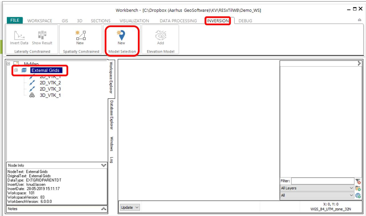
In the new window select which grid to turn into a model selection, it is possible to select more than one grid at a time by holding down the 'Ctrl' or 'Shift' key while selecting the grids.
