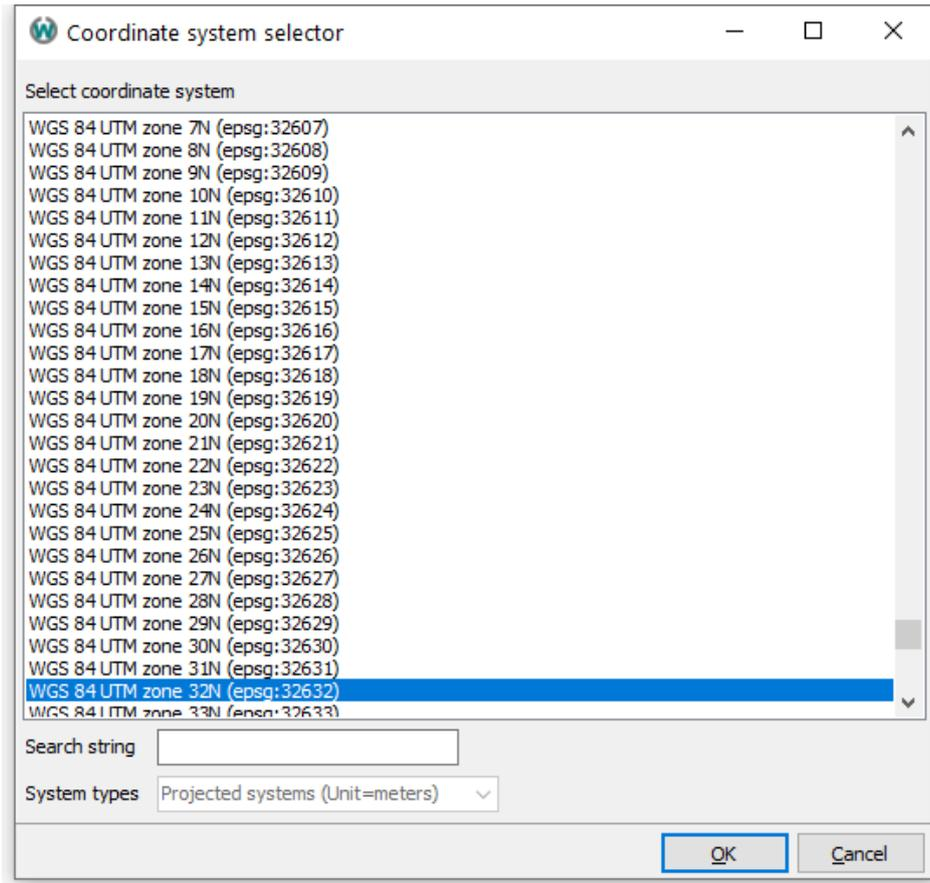
This must be the same as coordinate system as the global coordinates entered in the .dat file prior to inversion. Repeat this for all the VTK files you wish to import in the workspace.
