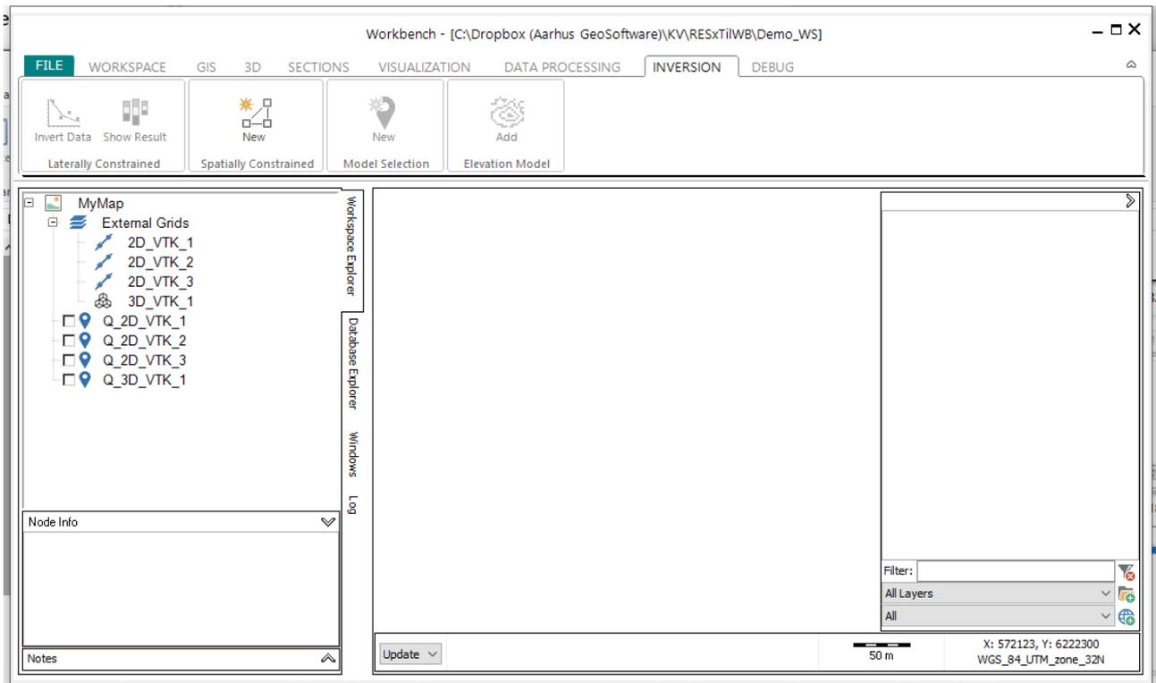
The different GIS/MAP layers can be toggled on and off in the GIS layer controller to the right on the screen, it is also possible to edit the order of the layers by dragging and dropping the layers in the GIS layer control. To add the locations of the models in the model selections to the GIS map check the checkbox next to the model selection in the Workspace Explorer, here an aerial photo and the three imported 2D inversions are shown on the map:
