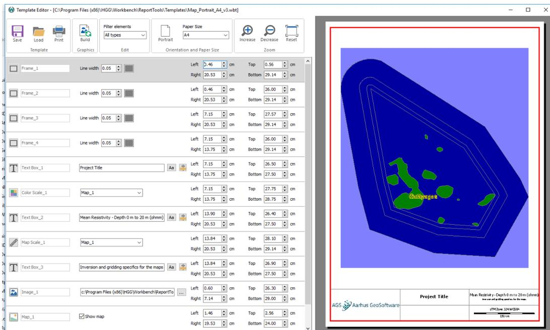
To the left the editor is shown, to the right a preview is displayed. It is possible to edit the size, location and appearance of each element. New elements are added by selecting the icon to the left of an element and selecting "Copy item". It is also possible to change the type of the element or to delete elements in this
