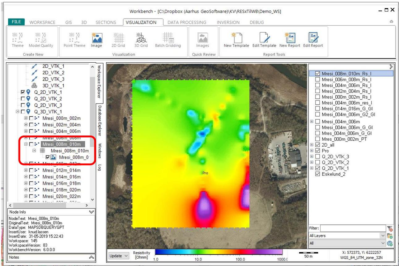
It is also possible to make 2D grids and images for several themes in a model selection in one go by highlighting the model selection and selecting “Batch Gridding”.
