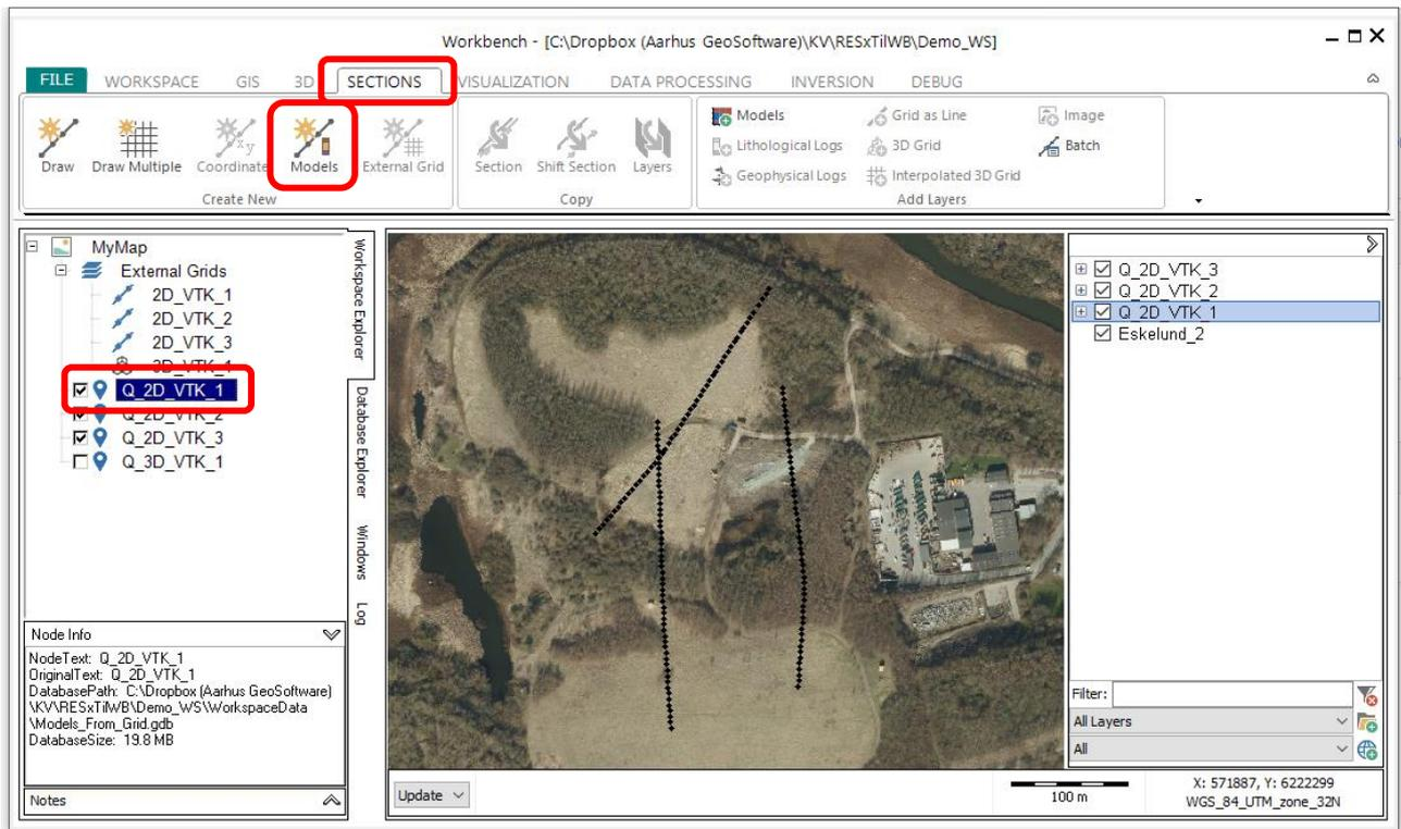
In the new window select the name and direction of the profile, as well as whether to plot results in resistivity or conductivity:
